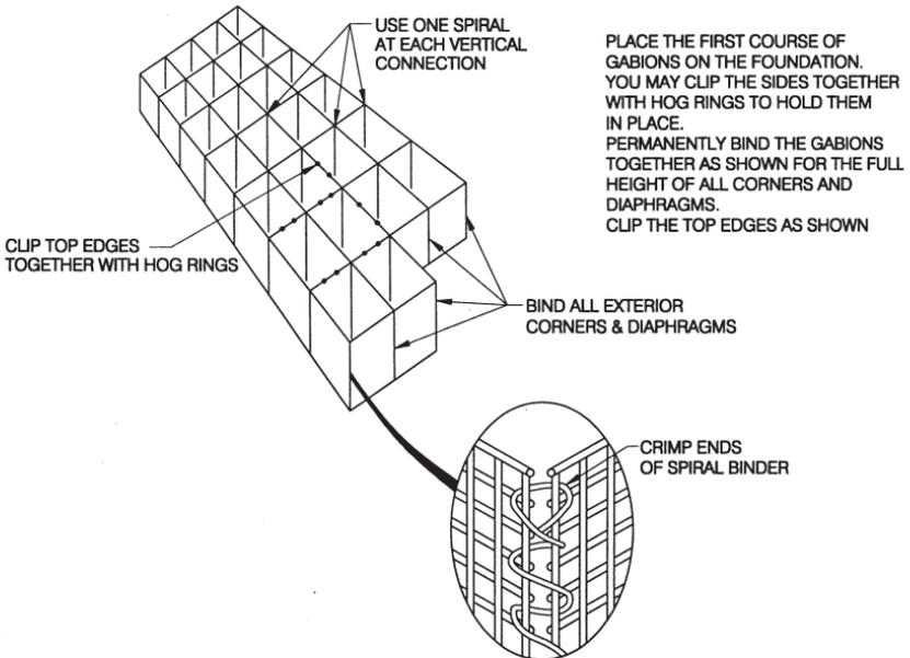
PLACE THE FIRST COURSE OF GABIONS ON THE FOUNDATION. YOU MAY CLIP THE SIDES TOGETHER WITH HOG RINGS TO HOLD THEM IN PLACE. PERMANENTLY BIND THE GABIONS TOGETHER AS SHOWN FOR THE FULL HEIGHT OF ALL CORNERS AND DIAPHRAGMS. CLIP THE TOP EDGES AS SHOWN
