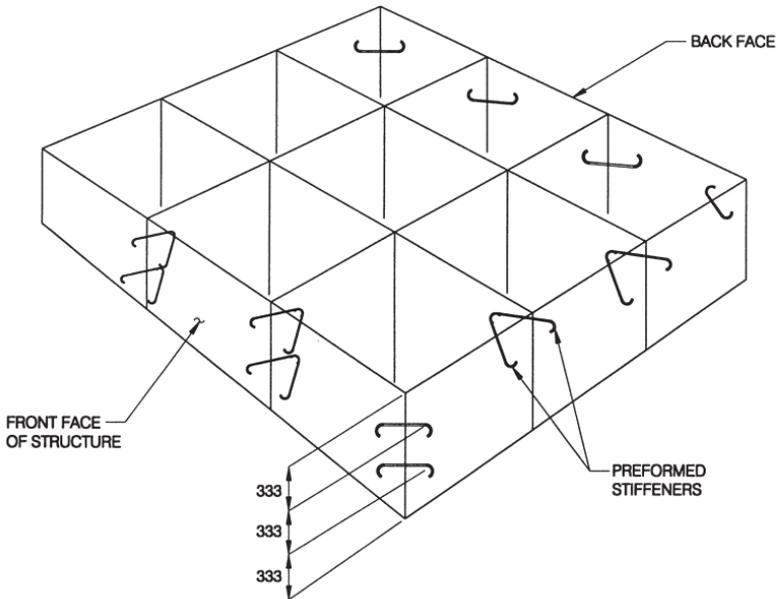
INSTALL PREFORMED STIFFENERS ACROSS THE CORNERS OF THE GABIONS BEFORE FILLING. TWO ROWS OF STIFFENERS (4 PER CELL) ARE REQUIRED ON THE FRONT FACE. INSTALL A SINGLE ROW (2 PER CELL) ON THE BACK FACE. NO STIFFENERS ARE REQUIRED IN THE INTERIOR CELLS.
