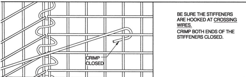
**Figure 13.8** Welded wire gabions preassembly.
