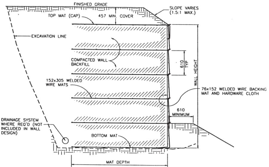
Figure 13.4 Welded wire wall.
