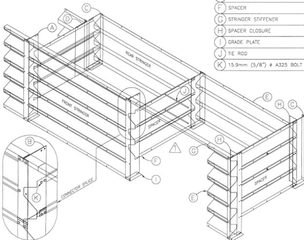
**Figure 13.3** Isometric view of Type III steel bin type wall
