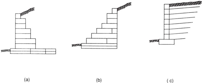
**Figure 13.5** Typical cross sections for a) gravity gabion wall (stepped); b) semi-gravity gabion wall; and c) reinforced soil gabion wall.
