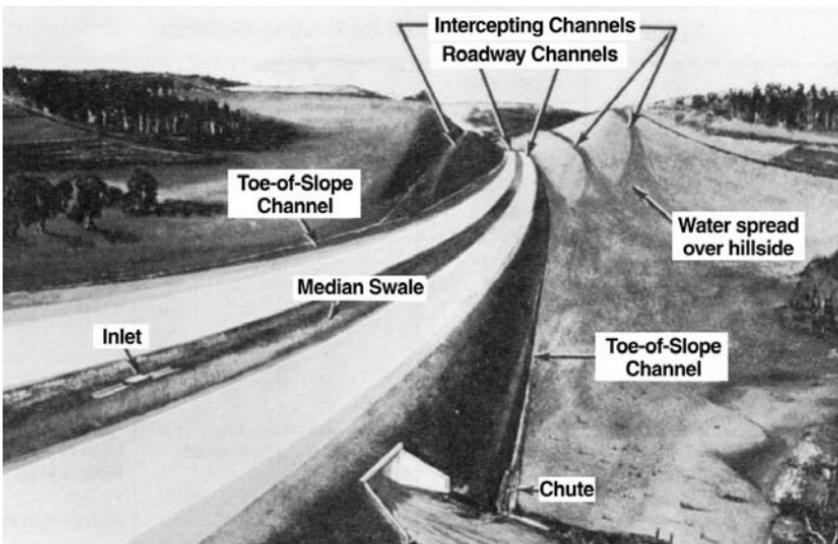
Figure 4.1 Types of roadside drainage channels.
