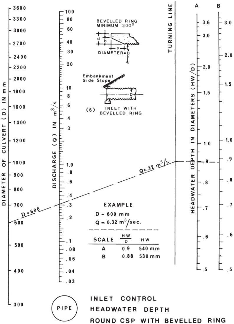
**Figure 4.11** Headwater depth for round corrugated steel pipe with bevelled ring under inlet control.
