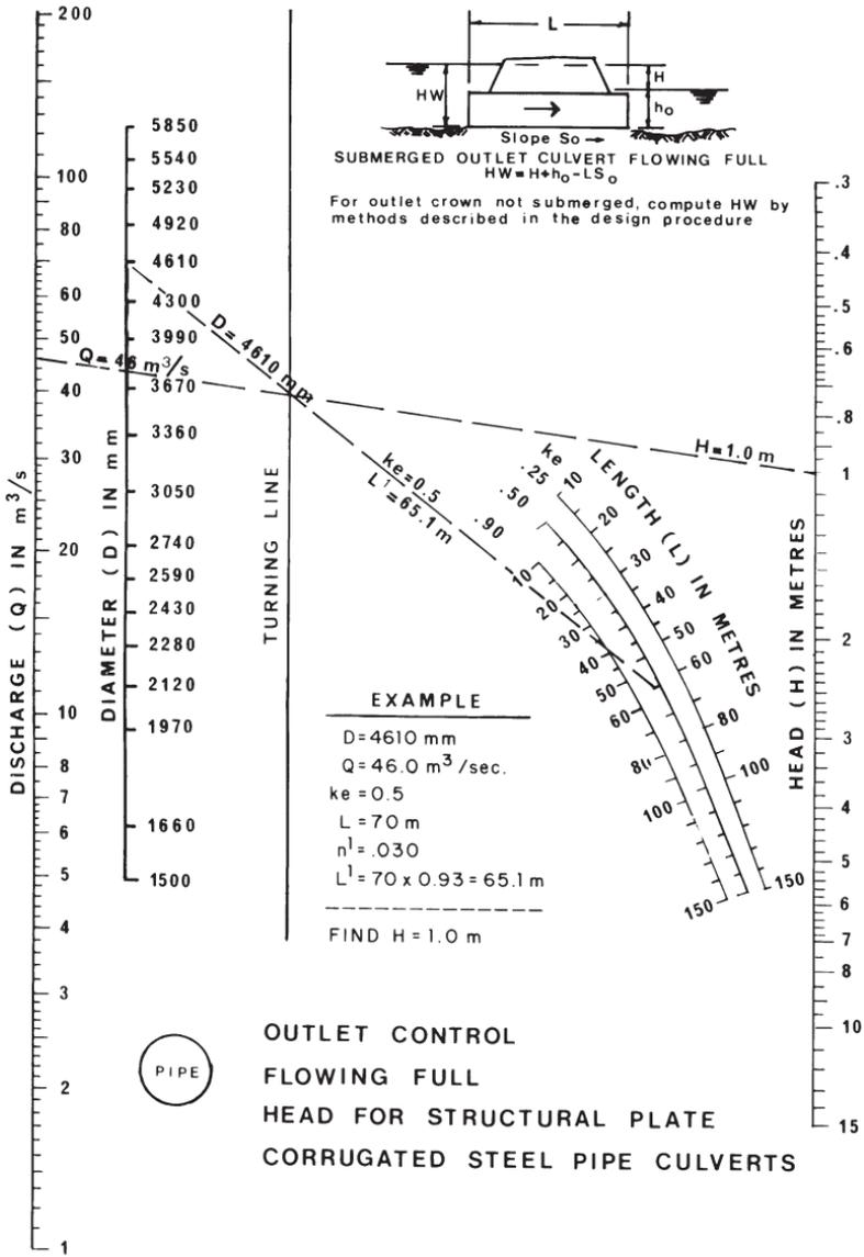
**Figure 4.18** Head for round structural plate corrugated steel pipe flowing full under outlet control.
