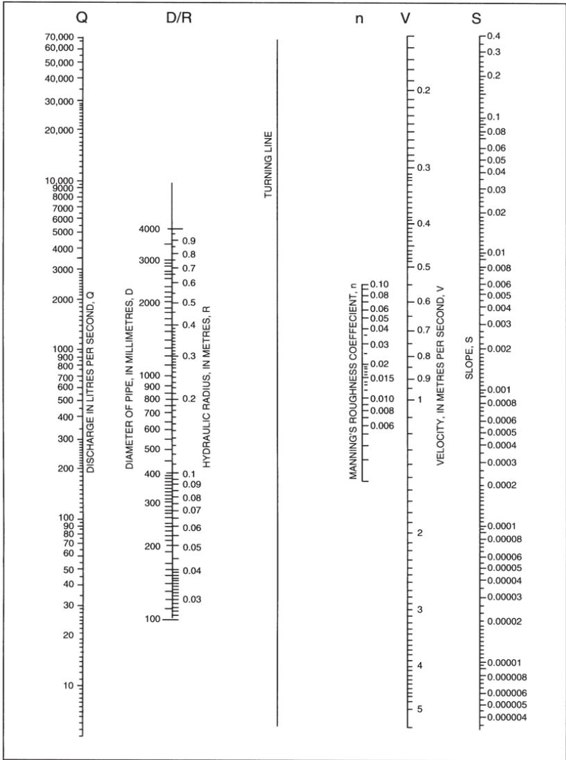
Alignment chart for energy loss in pipes, for Manning's formula.
