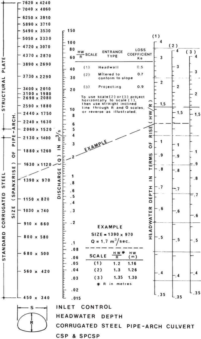
Figure 4.12 Headwater depth for corrugated steel and structural plate corrugated steel pipe-arch under inlet control.
