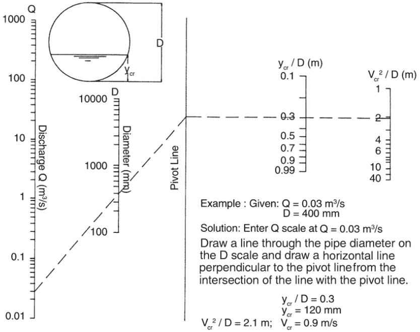
**Figure 4.25** Critical depth for round corrugated steel and structural plate corrugated steel pipe.
