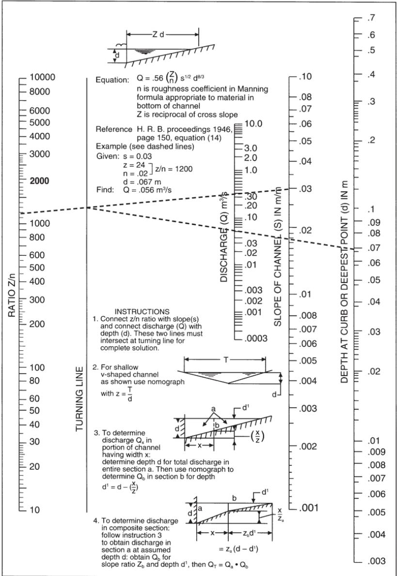
Figure 4.37 Nomograph for flow in triangular channels.
