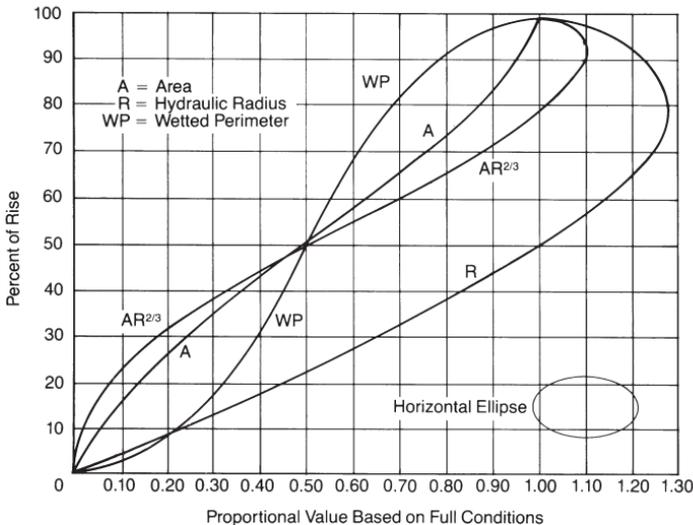
**Figure 4.30** Hydraulic properties of long span horizontal ellipse.
