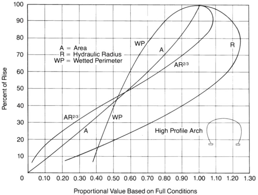
Figure 4.32 Hydraulic properties of long span high profile arch.
