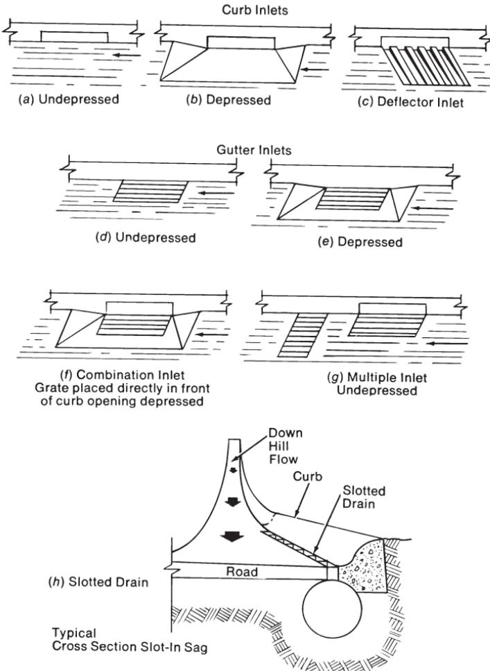
Figure 4.36 Stormwater inlets.
