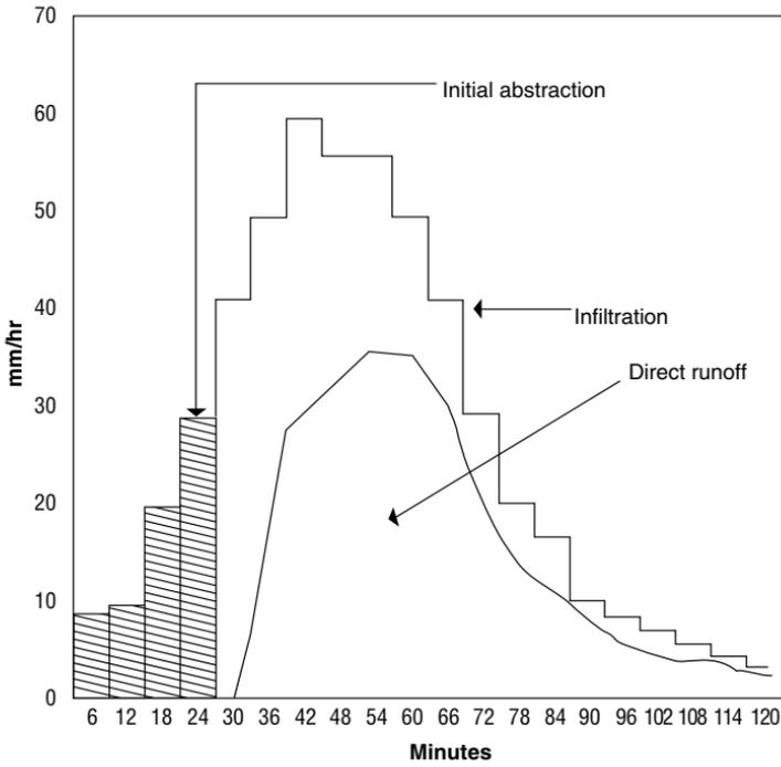
**Figure 3.9** SCS Method with  $I_a = 6.1$  mm and  $CN = 87.6$
