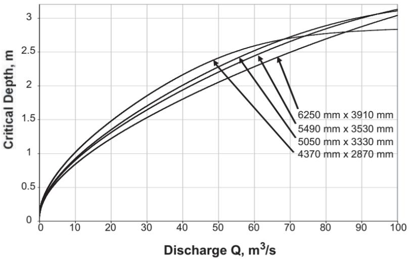
**Figure 4.27** Critical depth for structural plate corrugated steel pipe-arch.
