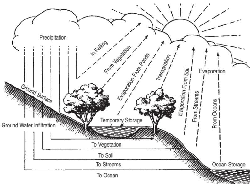
**Figure 3.1** Hydrologic Cycle - where water comes from and where it goes.
