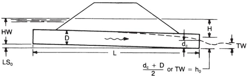
**Figure 4.9** Relationship of headwater to low tailwater.
