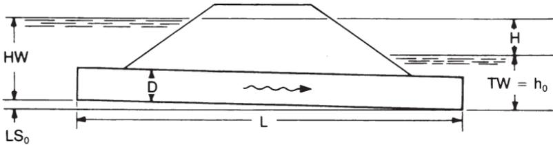
**Figure 4.8** Relationship of headwater to high tailwater.
