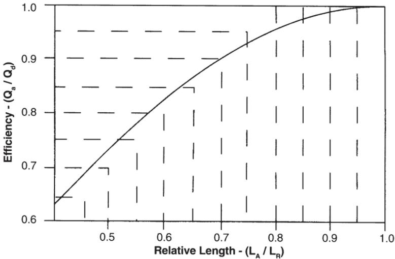
Example: if 20% carryover ( $Q_a / Q_d = 80\%$ ) is allowed, then only 58% ( $L_A / L_R$ ) of the total slotted drain length is required resulting in a 42% savings in material and installation costs.
