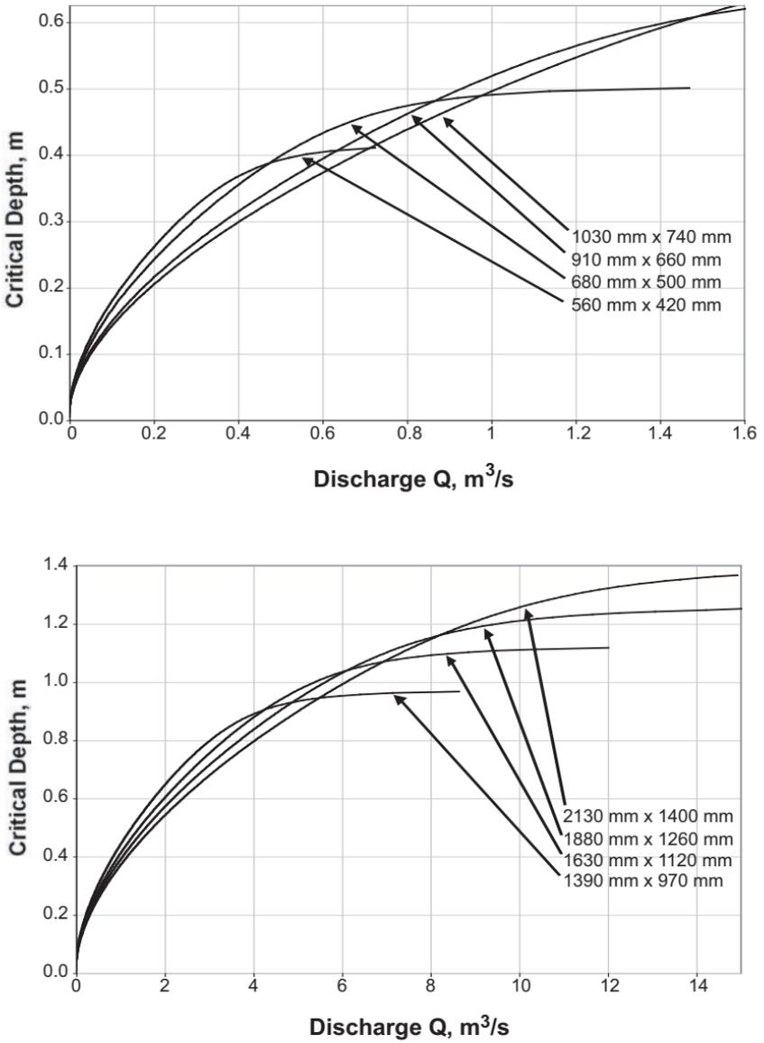
**Figure 4.26** Critical depth for corrugated steel pipe-arch.
