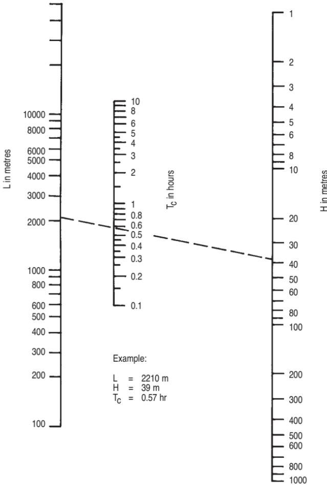
**Figure 3.11** T<sub>c</sub> nomograph using the Kirpich formula.
