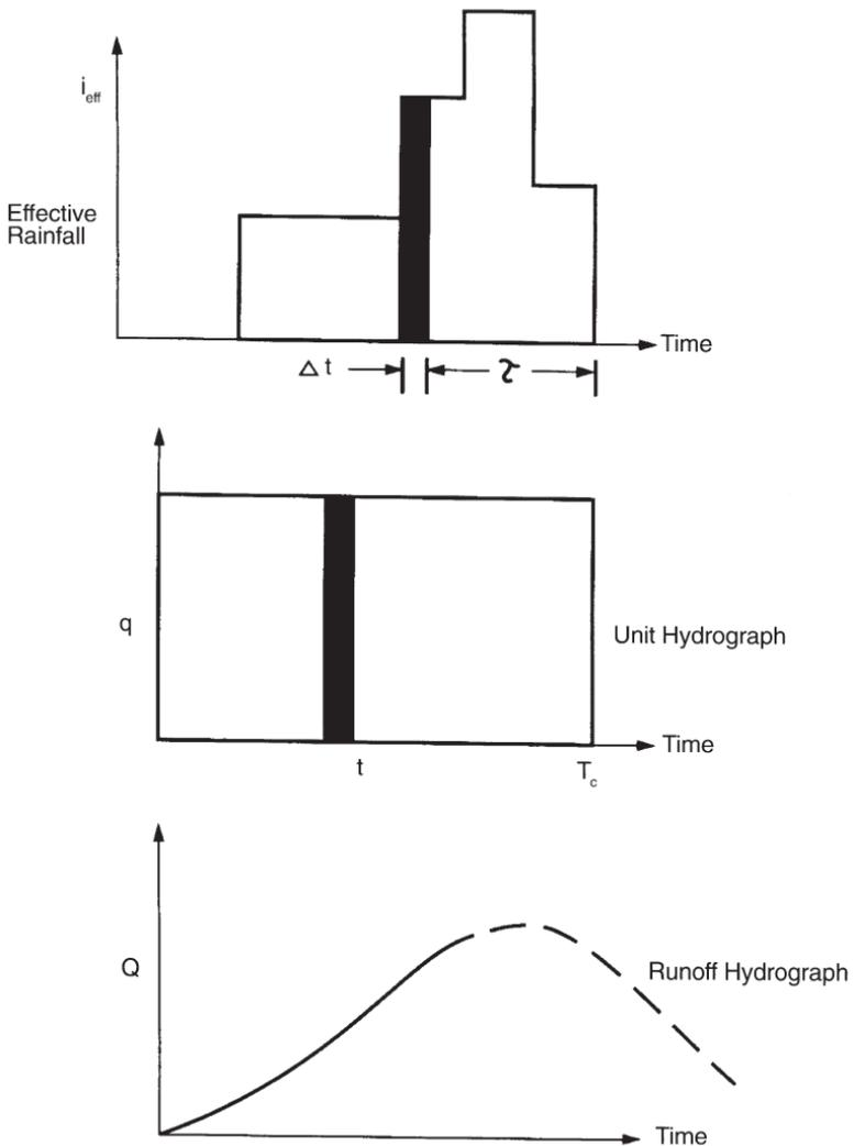
**Figure 3.15** Convolution process using a rectangular unit hydrograph.
