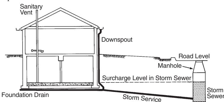
**Figure 2.1** Foundation drain and downspout connected to storm sewer by gravity
