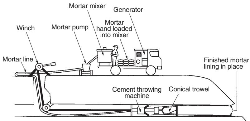
**Figure 11.5** Cement Mortar Lining
