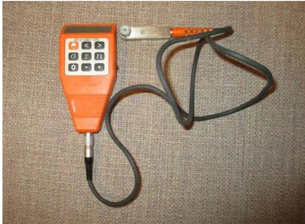
**Figure 3.** Elcometer 345 coating thickness gauge, with sensor facing upward at the end of an extension cable.
