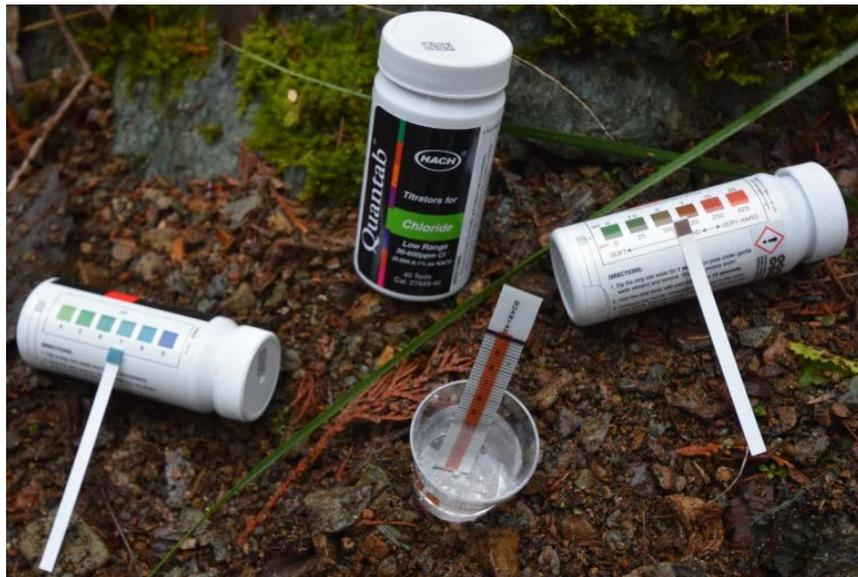
**Figure 1.** Colour indicator test strips for pH and total hardness, and a low-range chloride titrator (centre).
